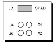
Figure 3 --- Enable scratchpad registers
